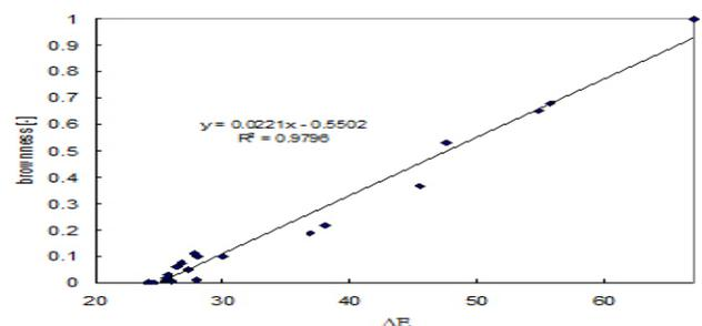
**Figure 7.** Correlation between brownness and measured  $\Delta E$  values
