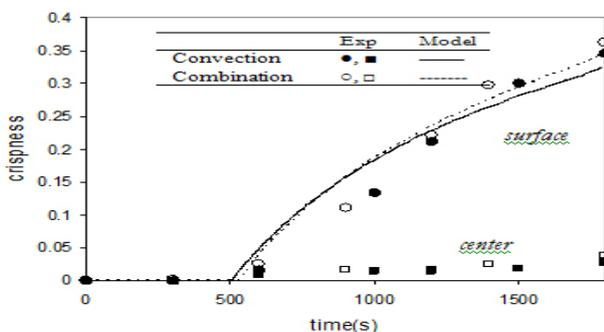
**Figure 10.** Crispness as a function of baking time. Experimental results (marker) and model simulation (line) for convective heating and combined heating inputs in the surface and center of product.
