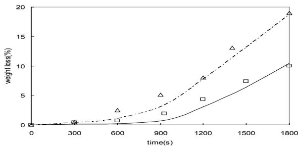
**Figure 4.** Product weight loss during baking with convective heating ( $\square$  : experiment; solid line: model) and combined microwave-convective heating ( $\Delta$ : experiment; dashed line: model).
