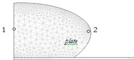
**Figure 2.** The product domain for simulation. Point 1 and 2 represent the center and surface points of the product for which the results are discussed (height 0.04 m, radius 0.04 m).
