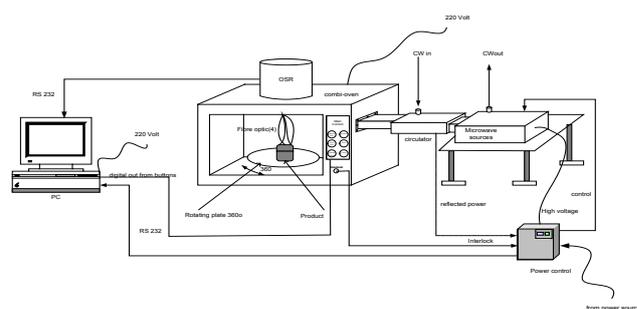
**Figure 1.** Equipment overview for baking
