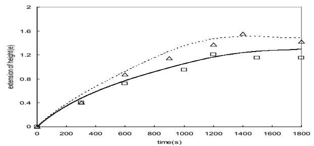
**Figure 5.** Height extension during baking with convective heating ( $\square$ : experiment; solid line: model) and combined microwave-convective heating ( $\Delta$ : experiment; dashed line: model).
