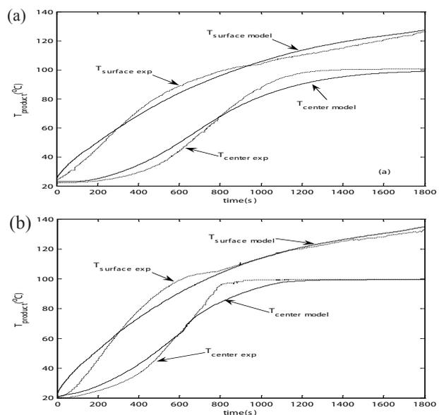
**Figure 3.** Product temperature during baking experiments (dashed line) and for model calculations (solid line) with convective heating (a) and the combination of convective and microwave heating (b).
